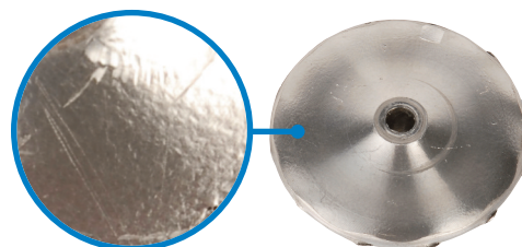
'Orange peel' effect on compressor wheels
